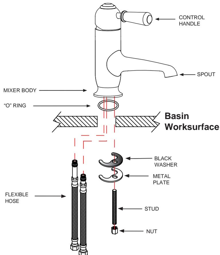
1. Fit the "O" ring into the groove on the underside of the mixer body.
